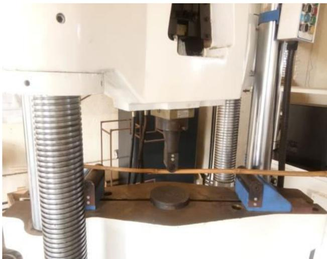
Fig -4: Hollow Cylindrical Bending Test
