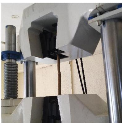
Fig -6: Bamboo Cylindrical Strip Tensile Test
