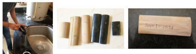
**Fig -2:** Treated and Untreated bamboo for water absorption test
