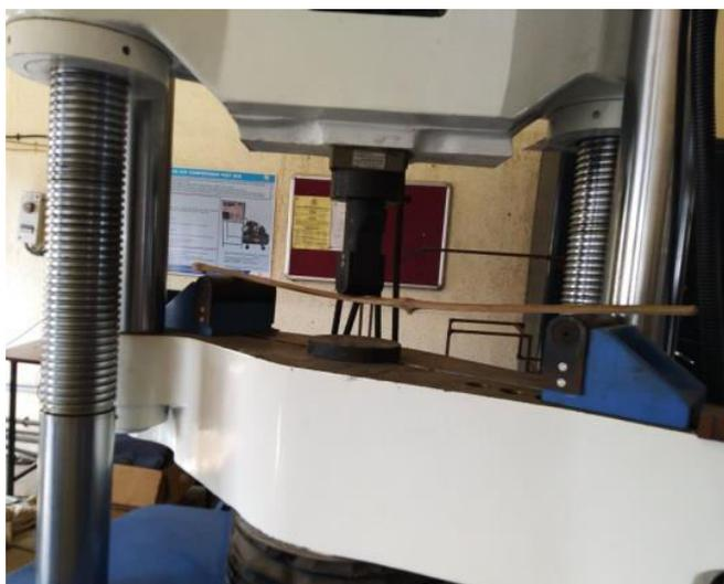
**Fig -3:** Bamboo Strip Bending Test
